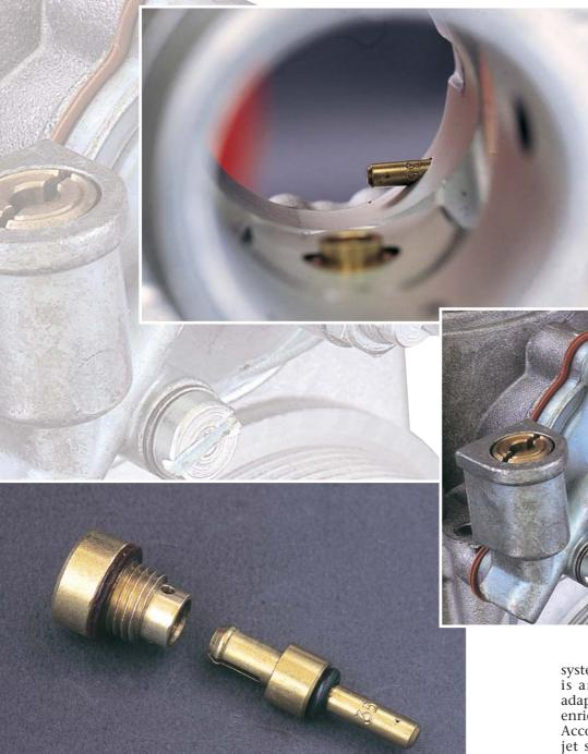
Below, the adjustment screw for the pump discharge allows adjustment of the flow. By turning clockwise the flow decreases, by turning
